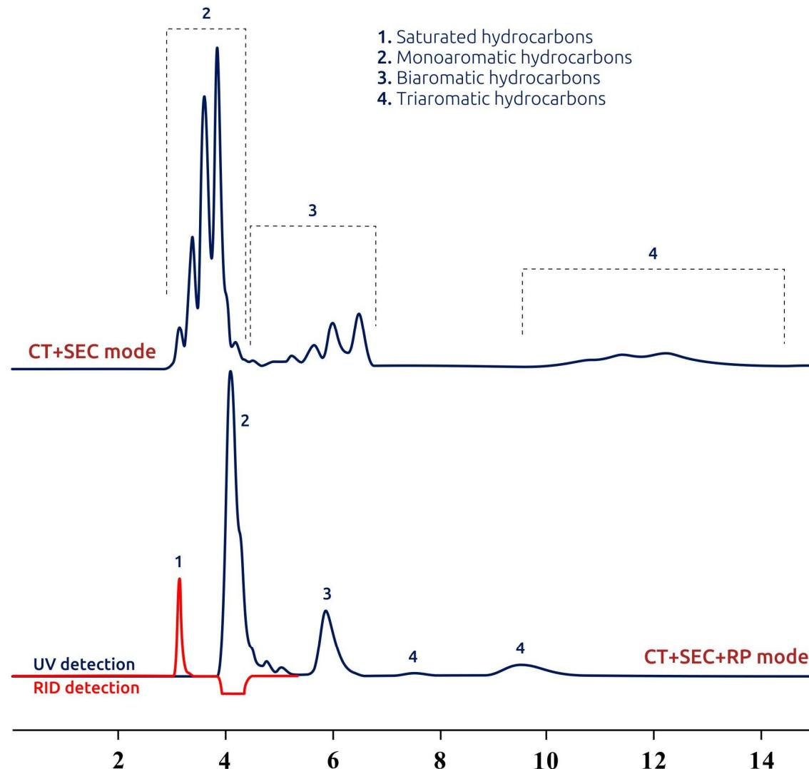
HPLC separation of petroleum aromatic hydrocarbons on NanoSpher Gasoline
